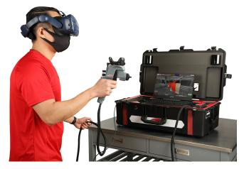
To shut down the unit, use the SimSpray menu in the upper left hand corner and select the Shutdown option. Confirm the shutdown (yes or no), and wait for the screen to go dark. For US units, the spray gun and HMD unit will automatically shut down with the SimSpray Go unit.
