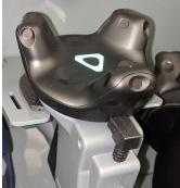
Press the blue triangular button on the top of the spray gun to turn on the gun; a green light will appear when the gun is on.
