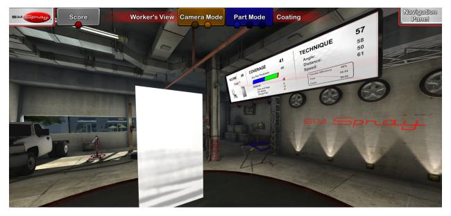
The coverage score also offers live insight into film thickness, defects like drips and sags, dry spray, and orange peel. The technique score offers live insight into angle, distance, speed, transfer efficiency, time spent in the booth, and costs.
