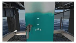
Point the spray gun at the option on the tablet and press the trigger to select and change the cue. Angle, distance, and speed cues show up in the virtual environment to guide the user's positioning and movements as they build muscle memory.
